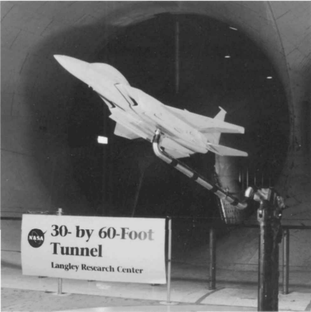
Fig. 5 10% scale F-15E model in NASA Langley 30-by 60-ft Wind Tunnel.
